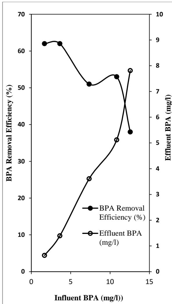
Fig.4. The Effect of Influent BPA on BPA Removal Efficiency(%)(COD:400-461 mg/l)
