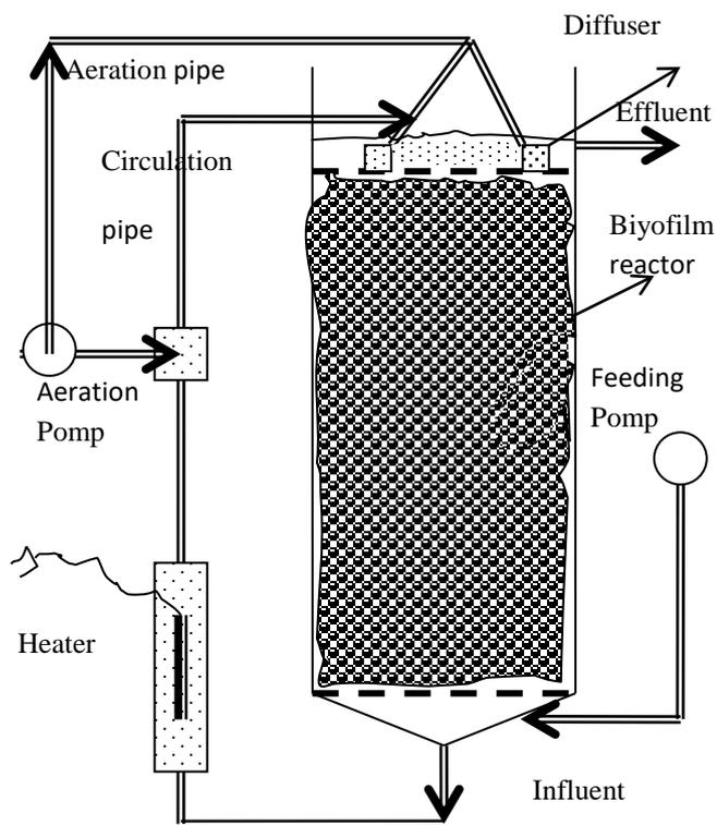
Fig. 1. Laboratory scaled biofilm reactor experiment apparatus
