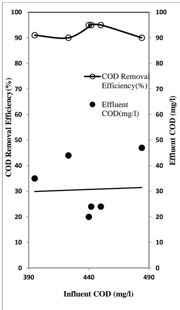
Fig.2. Effect of Influent COD Concentration on COD Removal Efficiency ( $\theta_h=6$  hour,  $pH:7$ ,  $T=25^\circ C$ )
