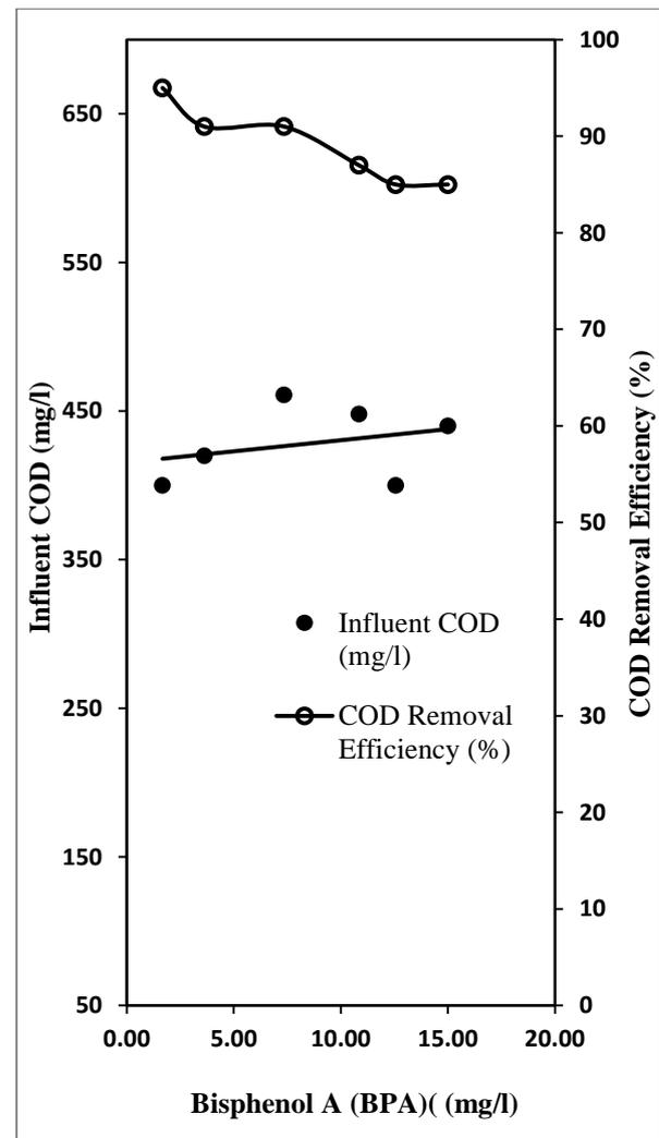
Fig.3 The Effect of Influent BPA Concentration on COD Removal Efficiency (%)
