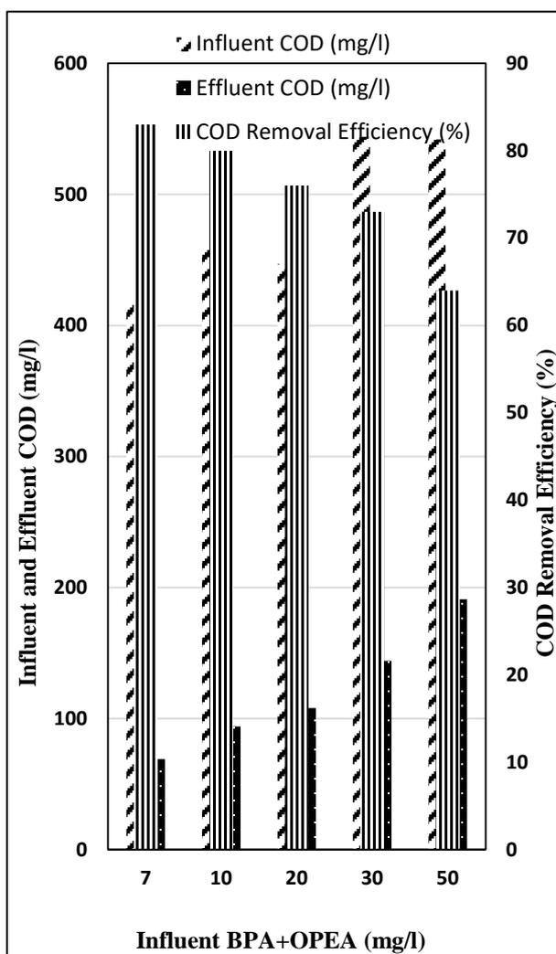
Fig.6. The Effect of BPA+OPEA Mixture on COD Removal Efficiency.
