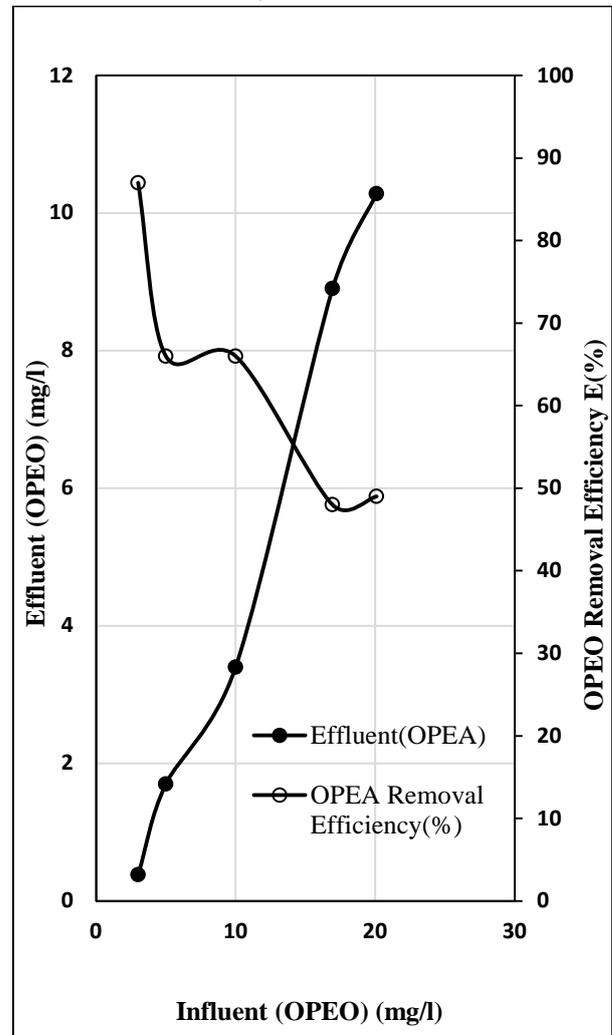
Fig.5. Effluent OPEA Concentration and OPEO Removal Efficiency Depending on the Influent OPEO (COD=450 mg/L)
