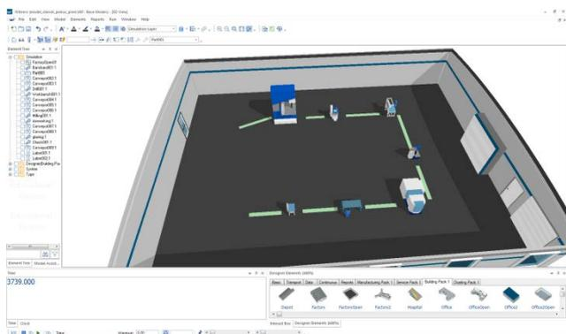
Figure 6. Model of production process - Witness 3D
