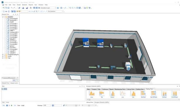
Figure 7. Model of production process after the optimization – Witness 3D
