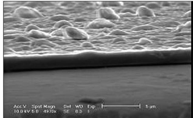
Figure 5. Image of a cross-section of a dental implant coating created by pulsed laser deposition technology [26]
