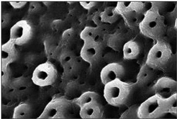
Figure 2. Application of anodic oxidation on the surface of dental implant TiUnite – Scanning Electron Microscopy, magnification 1400 [15]
