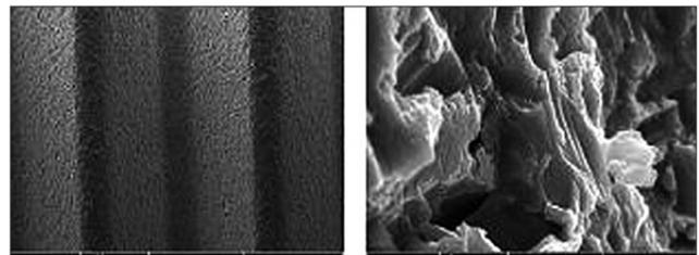
Figure 1. The surface area of titanium implant sandblasted with  $\text{TiO}_2$  particles - Scanning Electron Microscopy, magnification 100 (left) and 7500 (right) [11]
