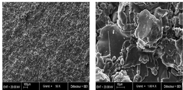
Figure 4. Dental implant surface after the application of titanium plasma spraying [11]
