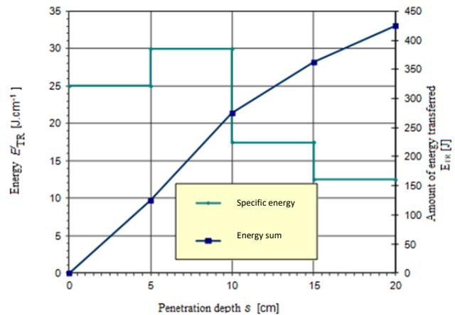
Figure 5. Transmitted energy ( $E_{TR}$ ) and transmitted energy per gelatin trajectory function of the offending section of the bullet trajectory in the gelatin block. (Source: [3])
