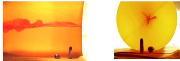
Figure 2. Shape of the temporary cavity defined by the system of radial ruptures after the penetration of the gelatine block by a 9 mm Luger Gold Dot pistol cartridge bullet (Left – horizontal cut of the block at the wound track location, right - view of the cross-section front with star-shaped radial ruptures) (Source: [3])
