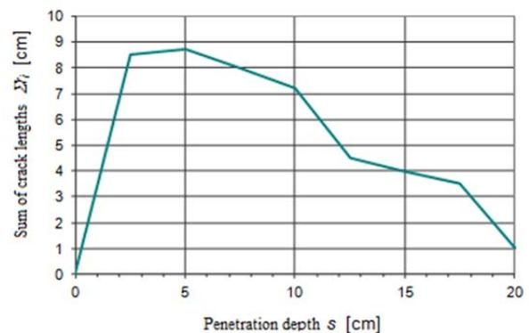
Figure 3. Diagram of the dependence of the sum of ruptures lengths  $\Sigma r_i$  on the depth of a bullet penetration into a gelatin block (Source: [3])
