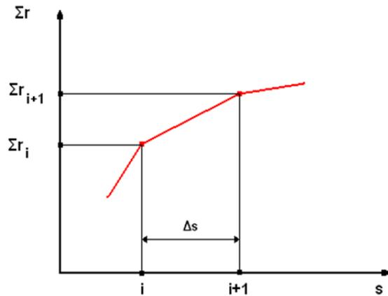
Figure 4. Construction of the dependence of the total length of radial ruptures on the bullet trajectory (Source: [3])
