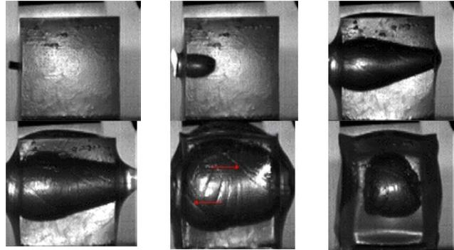
Figure 6. A series of selected images from the continuous recording of the gelatine block penetration with an bullet of a calibre 40 S & W (frame rate 20,000 sn.s<sup>-1</sup>)
