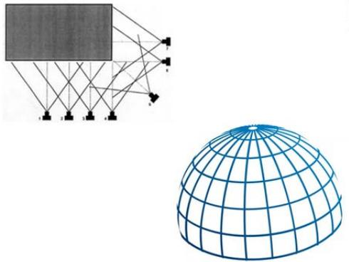
Figure 13. How to take photos for a photogrammetric survey which overlap each other and form a virtual sphere around the object
