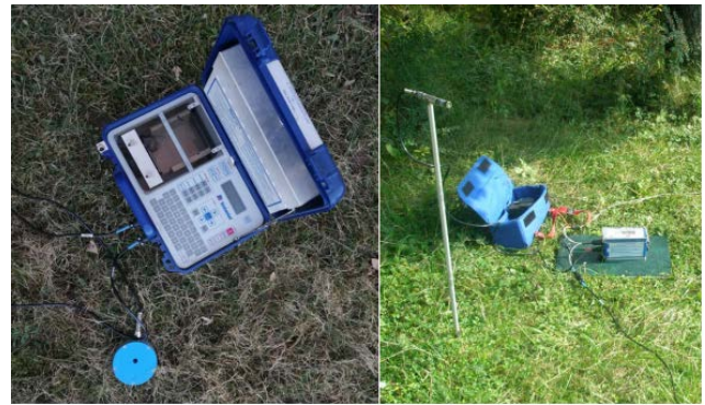
Figure 1. Blastmate III and Minimate Plus seismographs
