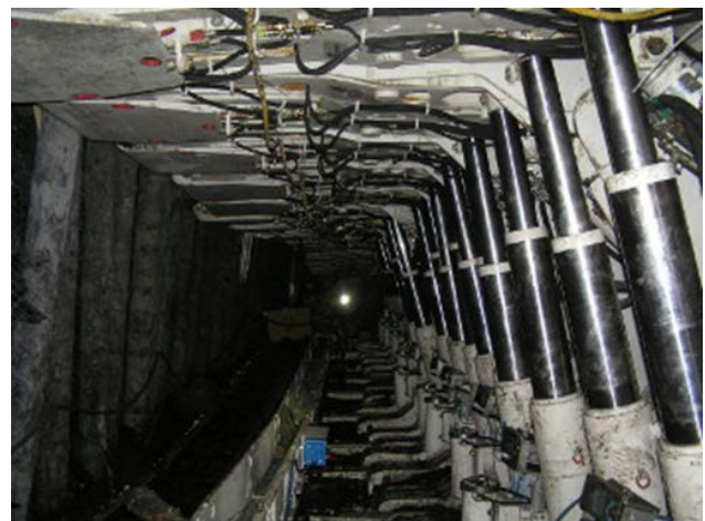
Figure 3. Cross-section of a mechanized longwall face opening
